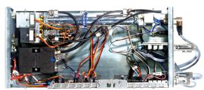
Interior view, showing one NDIR, one NDUV bench, one paramagnetic  $O_2$  cell, analog and relay outputs, digital inputs, and serial interface.
