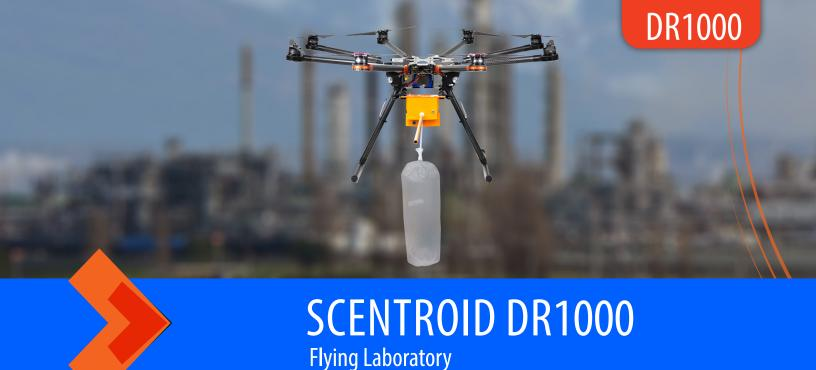
he Scentroid DR1000 consists of a flying laboratory and a commercial drone. The DR1000 can be used to sample and analyze ambient air at heights of up to 150 meters above ground level that was previously impossible to accomplish. Air quality mapping, model verification, analysis of potentially dangerous sites are all made possible by this novel innovation.
