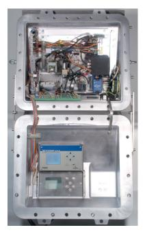
Interior view, showing one NDIR bench, one NDUV bench, one paramagnetic  $O_2$  cell, thermostatic control (cover removed), analog and relay outputs, digital inputs, and a serial interface.
